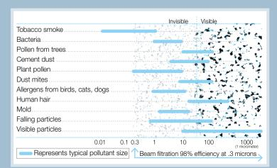
It starts by taking the dirt out of the house directly to the power unit collection canister using cyclonic forces to separate larger dirt particles and allergens from vacuumed air. Then it removes tiny particles at .3 microns with a permanent HEPA-filtration material.
